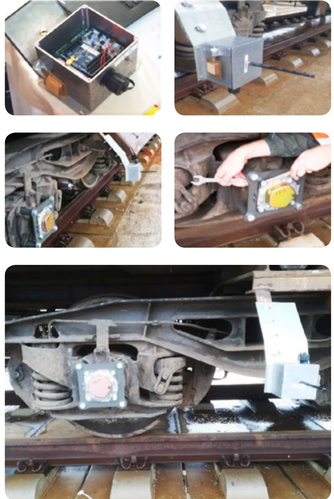
↑ FIGURE 17 OTI components Installation in Relevant Environment
