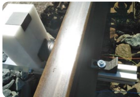
FIGURE 10 Variable Reluctance Energy Harvester (non-contact). 10W Theoretically output peaks during wheel passing, , around 250mW average power.
