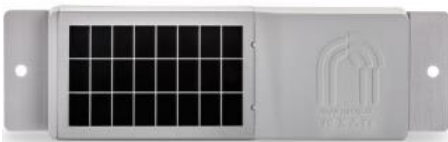
Figure 14 - Nexiot Solar Powered Tracking Device
