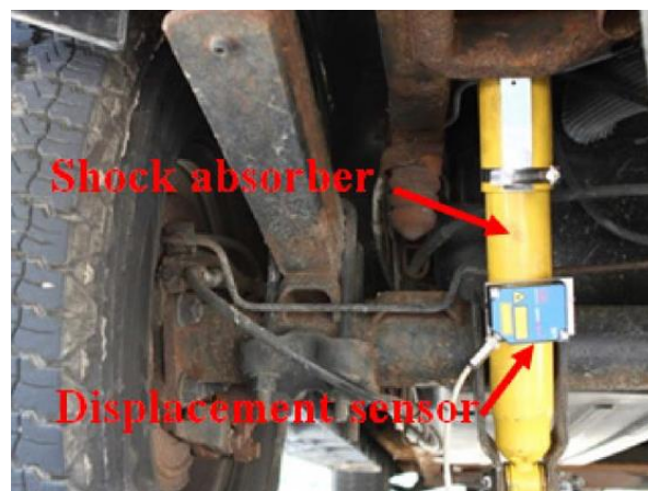
(c) Experiment setup for suspension vibration tests
