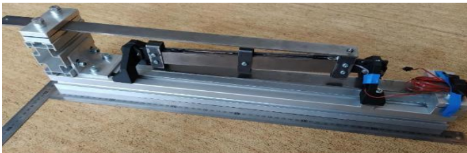
Passive – harvests waste energy through vibration
