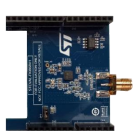
COM module (S2-LP board)
