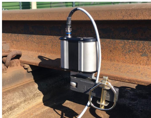
Fig. 51 ReVibe energy harvester mounted on track. [66]
